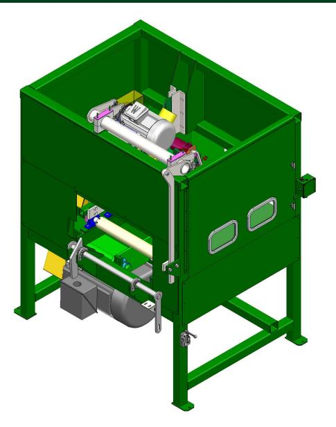
The Pendu Lineal Dap Notcher daps the top and bottom of crossing panels for a snug fit to the rail. Designed to run at a max speed of 40 feet per minute, the Lineal Notcher can produce 900 single pieces a day using 12' long material. The Lineal Notcher also features top powered hold down rolls and a Hyd drive.
