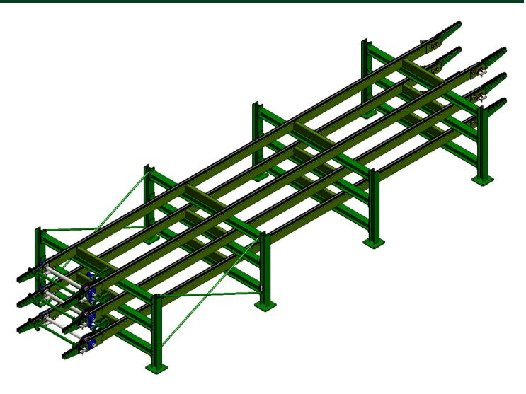
Pendu Railway Tie Sorting Decks collect ties from your production line and sorts them onto multiple levels. 35' long accumulator chains hold approximately 77 ties at a time.
