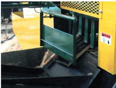
Heavy 1/2" plate steel fingers help hold smaller pieces of wood securely.
